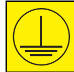
PESC-†-EC Protective Earth (Ground)
