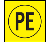
PESC-†-PE Protective Conductor
